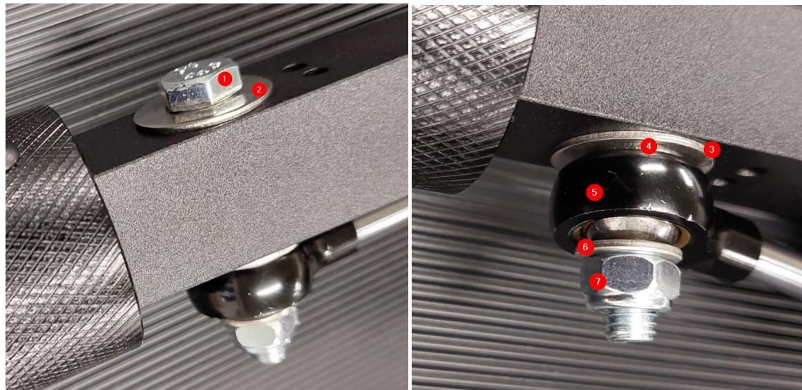
The bottom attachment is made in one of the collective arm slots using the M4x40mm socket screw.
